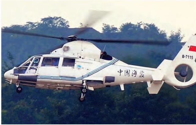
Photo 13. A helicopter operated by China Maritime Surveillance. This is a type Z-9 design that is used widely among China's armed forces. (China Defense Forum)
