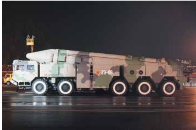
DF-21C ballistic missile preparing for 1 October 2009 parade in Beijing. An anti-ship ballistic missile would be based on a variant of the DF-21 ballistic missile. The transporter-erector-launcher (above) allows for mobility and makes targeting by enemy forces harder.
