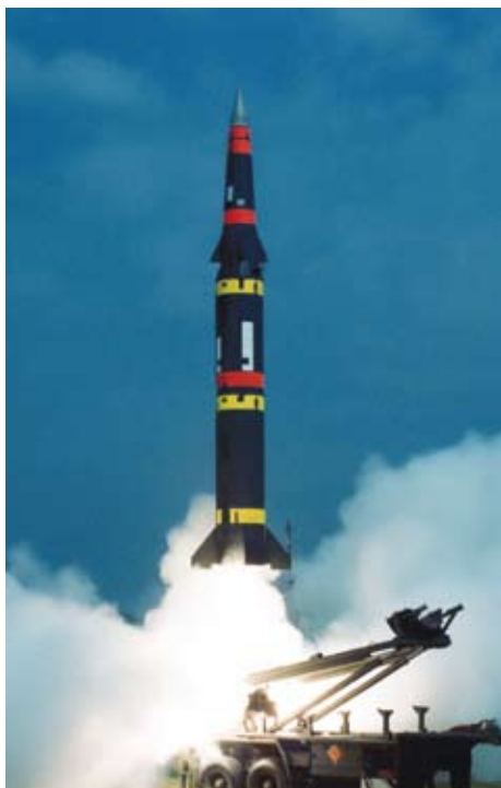
A FAMILY RESEMBLANCE? According to Chinese sources, a DF-21/CSS-5 ASBM would be based on the U.S. Pershing II (left), as is the DF-15/CSS-6 missile (right). The Pershing II has adjustable second stage control fins for terminal maneuver. While the DF-15 pictured here lacks similar control fins, one with a reentry vehicle virtually identical to the Pershing II's may be found at http://www.sinodefence.com/strategic/missile/df15.asp .
