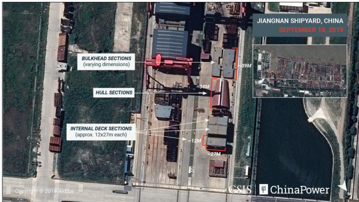
Figure 11. Type 002 Aircraft Carrier Under Construction
