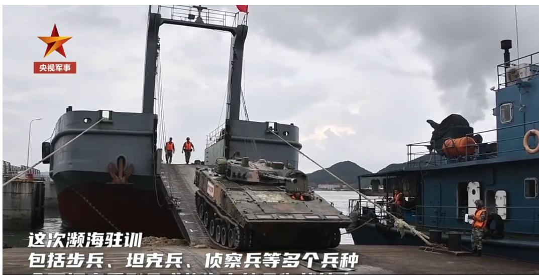
Figure 4. Bow ramps on deck cargo ships allow for easy loading and unloading as shown here in the 2021 training exercises. 12
