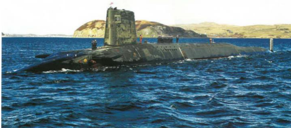
The huge side sonar array of the British "Vanguard" class strategic nuclear submarine is striking
