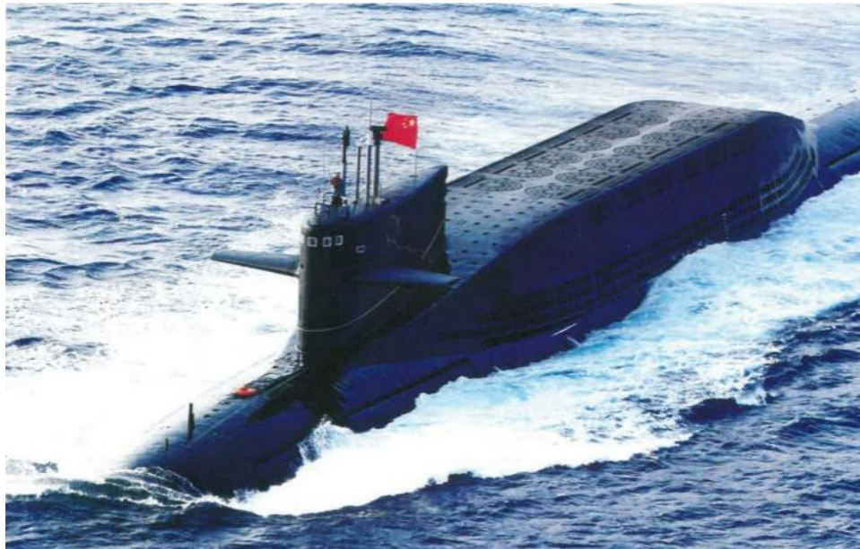
The Type 094 strategic nuclear submarine is equipped with 12 missile tubes and can load 12 Julang-2 missiles
