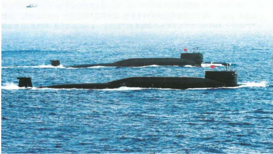
Two Type 094 strategic nuclear submarines are sailing side by side. There are subtle differences in the command platform enclosures of the two boats, indicating technical improvements have been made.
