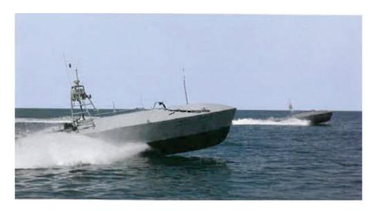
The US military's general-purpose USV was jointly developed by AAI Unmanned Aircraft Systems and Textron Systems and was put into use in 2012. This type of vessel adopts a modular design and has a powerful payload. It can detect mines in patrol waters through the side-scan sonar installed on the boat and transmit relevant data back to the mother ship through the communication equipment on board. It also has unique advantages in data links and fuel, and is efficient, high-speed, and safe.
