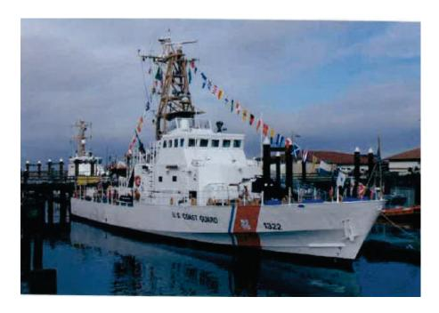
The *Island*-class patrol boats were built between 1985 and 1992 with a total of 49 completed. The vessel is 34 meters long, has a displacement of 168 tons, a maximum speed of 53 km/hr, and a self-sustaining capacity of five days. It is also equipped with a 25mm gun, two 12.7mm machine guns, and AN/SPS-73 radars capable of tracking up to 200 targets. However, the Island-class is currently being replaced by the Sentinel-class fast response patrol boats.
