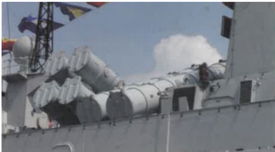
Two quad-mounted “Yingji” [YJ]-62 anti-ship missile launchers on the Type 052C destroyer.
