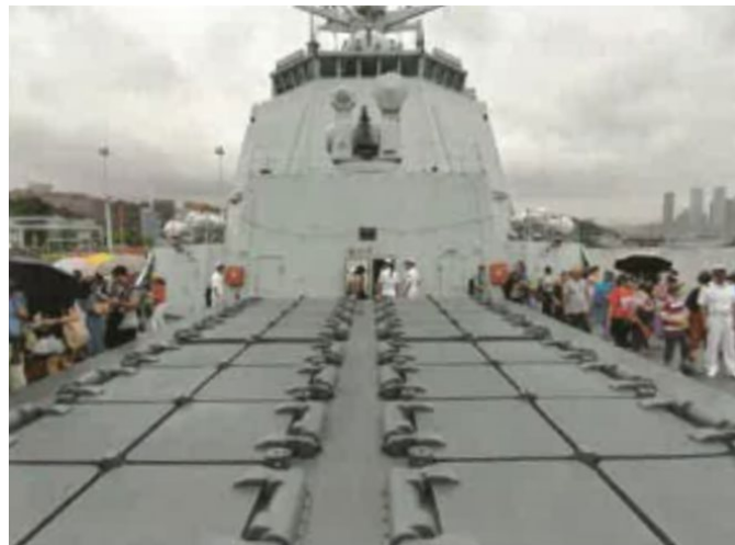
Missile vertical launch system at the forward of the Type 052D destroyer.
