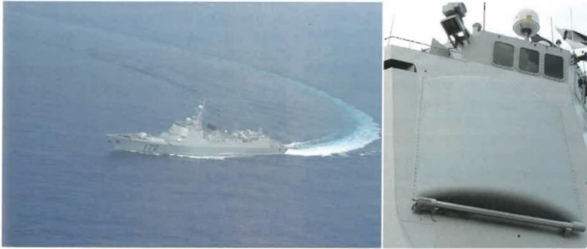
The "Lanzhou" is conducting tactical maneuvers at sea. Its black hull number shows that it is in its early service state. A close-up of the antenna array of the active phased array radar of the Type 052C destroyer (right picture).
