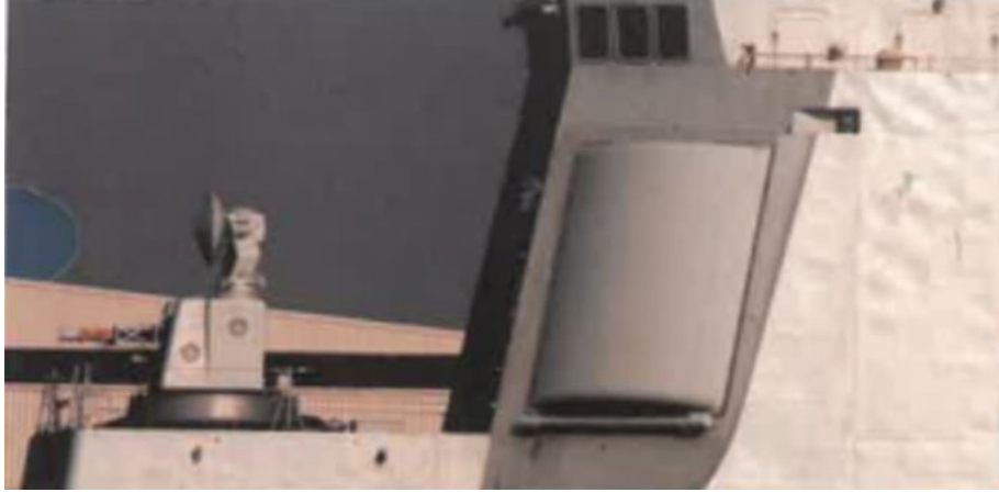
The active phased array radar of the Type 052C may be the focus of the Type 052C destroyer modification and upgrade.
