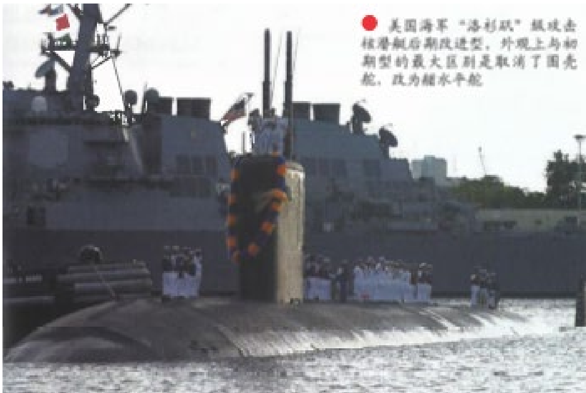
A later flight, improved U.S. Navy Los Angeles -class nuclear-powered attack submarine. The biggest external difference from the earlier flight was the removal of diving planes from the sail, placing them on the bow.
