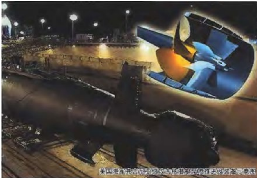
Figure 4: Schematic diagram of pump-jet propulsion and equipment of the U.S. Navy Virginia-class nuclear attack submarine.
