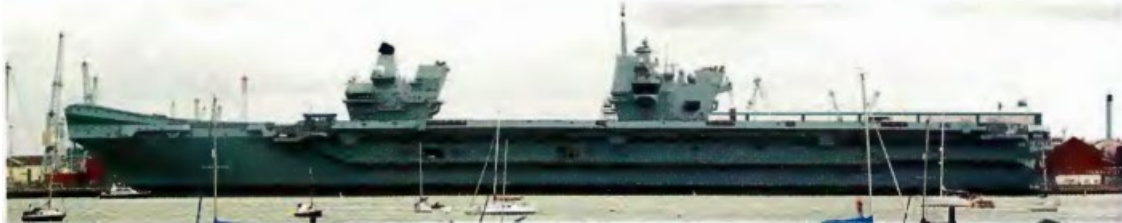
Side view of the British Royal Navy's Queen Elizabeth aircraft carrier, showing the considerable distance between the twin islands
