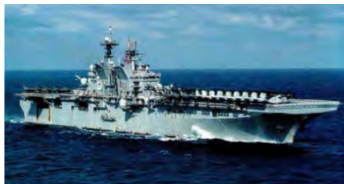
The USS America amphibious assault ship of the U.S. Navy features a large, cluttered single island with a substantial radar cross-section, which is highly detrimental to its stealth capabilities
