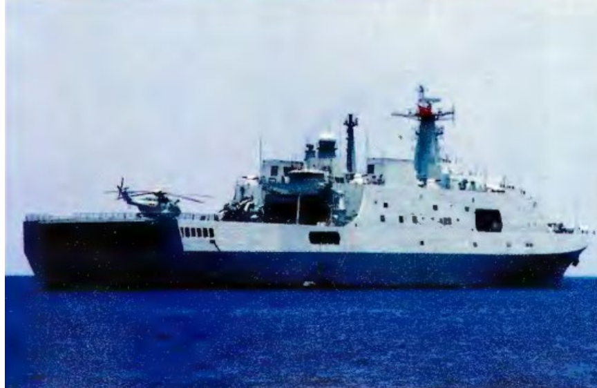
The stern of the Chinese navy's Type 071 dock landing ship features a hangar and flight deck and is capable of accommodating four large helicopters
