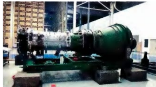
The GT-25000 gas turbine engine is powerful and an excellent naval propulsion system
