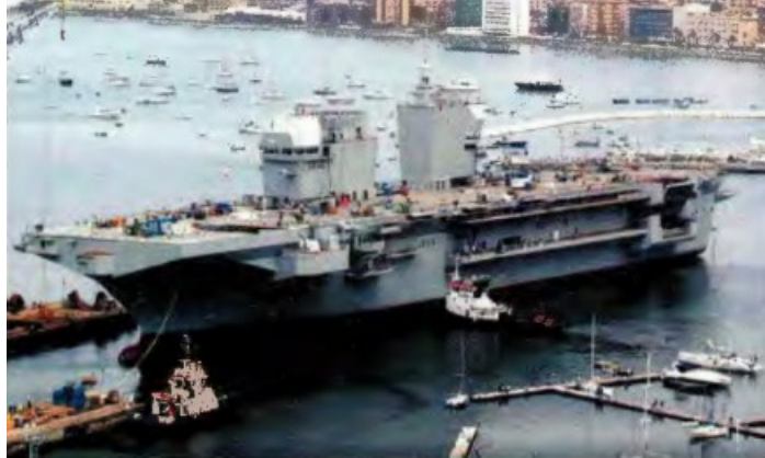
The Italian Navy's amphibious assault ship Trieste also employs a twin-island design
