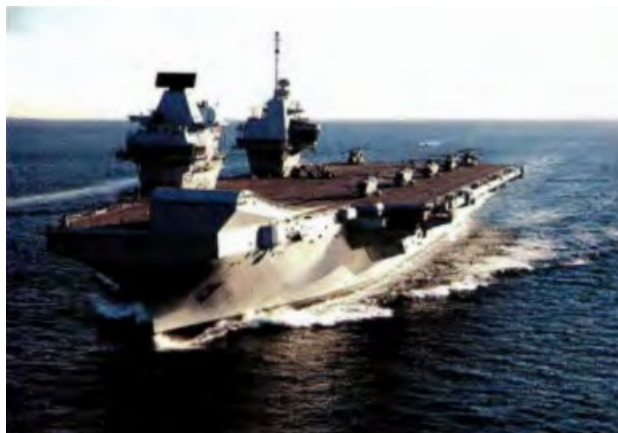
The British Royal Navy's Queen Elizabeth aircraft carrier adopted a twin-island design
