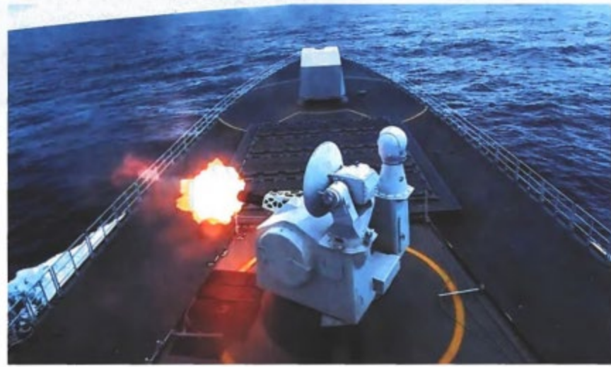
The Zunyi warship firing its close-in weapon system.
