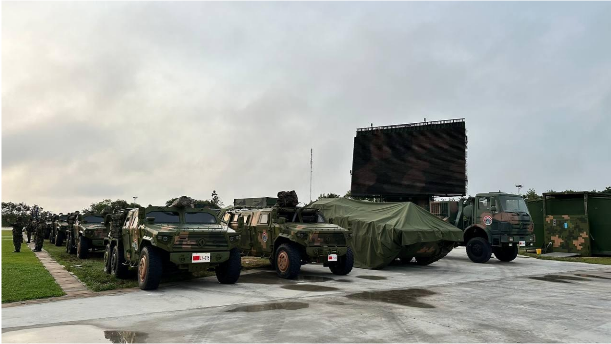
Figure 13. Cambodian news video of PLAA (from left to right) PCL171 122mm wheeled high-mobility howitzers, CSK181 wheeled light high-mobility assault vehicles, ZBD04A tracked IFVs (covered), and a YLC-2V long-range 3D air surveillance radar detachment; all vehicles were transported on PLAN lift for Golden Dragon-2025 . 39
