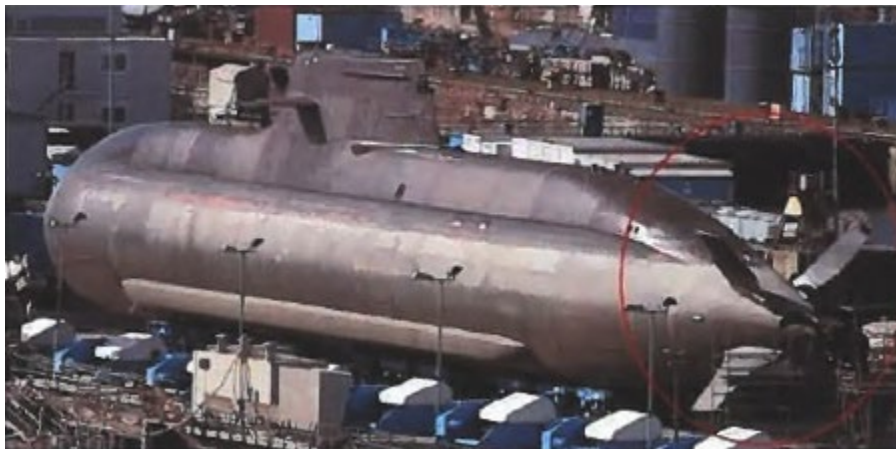
The X-shaped stern rudder is better suited for high-power “small-reactor” AIP systems.
