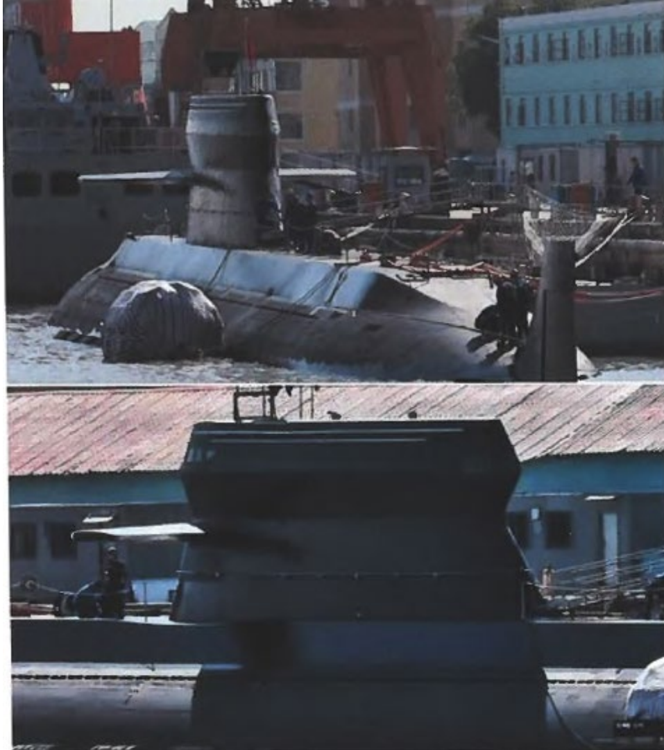
Foreign media has observed that the sail of China's new conventional submarine resembles that of the latest improved Type 039 variant, yet there are significant differences in the stern rudder and the submarine's length (see top and bottom images).
