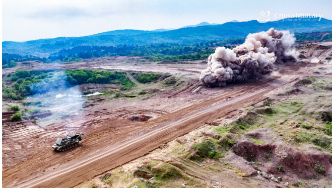
An integrated minesweeping vehicle attached to an engineer element of a combined-arms brigade under the Chinese PLA 71st Group Army detonates explosives during a minesweeping operation on April 9, 2025. (eng.chinamil.com.cn/Photo by Lin Weihong)
