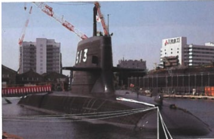
Image 9: In the latest Taigei-class submarines, the Japan Maritime Self-Defense Force has, for the first time, replaced lead-acid batteries and the Stirling AIP system with lithium-ion batteries. This gives the submarine strong low-speed submerged endurance and high-speed underwater performance, while also delivering a significant improvement in acoustic quieting.
