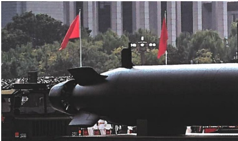
Image 19: The new generation of large unmanned underwater vehicles displayed in the September 2025 military parade already adopted an X-rudder design and a pump-jet propulsion system, which from another angle shows that both technologies have become highly mature in China. Their widespread use on the new submarine presents no technical obstacles whatsoever.
