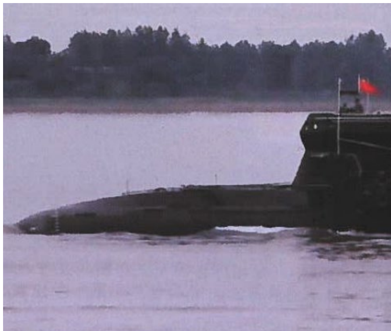
Image 16: Detail view of the 039C's bow and axe-type sail.
