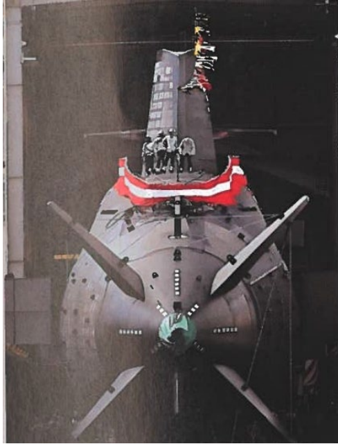
Image 17: X-rudders are now widely adopted on modern submarines; the Sōryū and Taigei classes both employ them. This image shows a close-up of the Taigei's X-rudder
