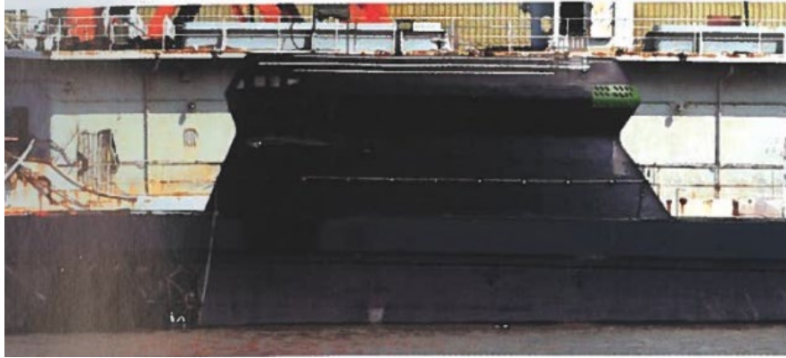
Image 12: Although the axe-type sail concept was first proposed by Sweden and adopted on its next-generation A26 submarine, delays in the A26 program mean that the 039C ultimately pulled ahead, becoming the first submarine in the world to be fully built and commissioned with an axe-type sail.
