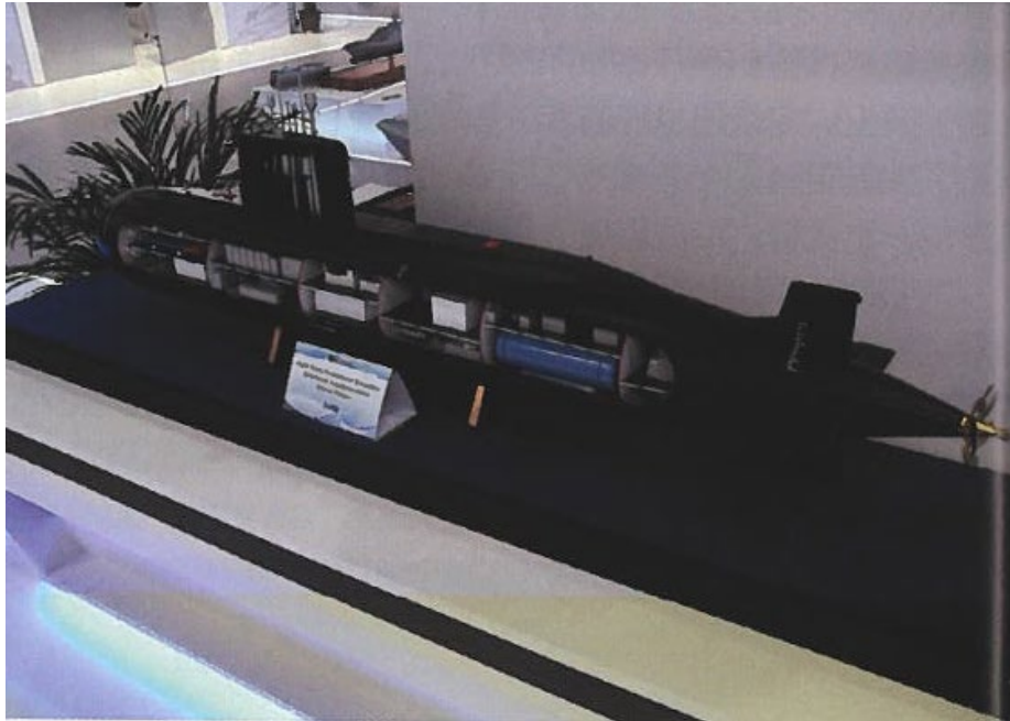
Image 33: China's S20 conventional submarine, offered on the international market, uses a Stirling AIP system (with a streamlined stern section for integration, a high-efficiency cooling/heating system, and a lightweight radiative cylindrical liquid-oxygen tank). It has already been exported to Pakistan
