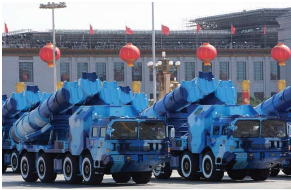
People's Liberation Army trucks carrying DH-10 land-attack cruise missiles drive past Tiananmen Square in Beijing during a parade marking China's 60th anniversary, 1 October 2009. China's estimated 150 to 350 DH-10s can use a variety of guidance systems and satellite inputs to achieve an accuracy of 10 meters.
