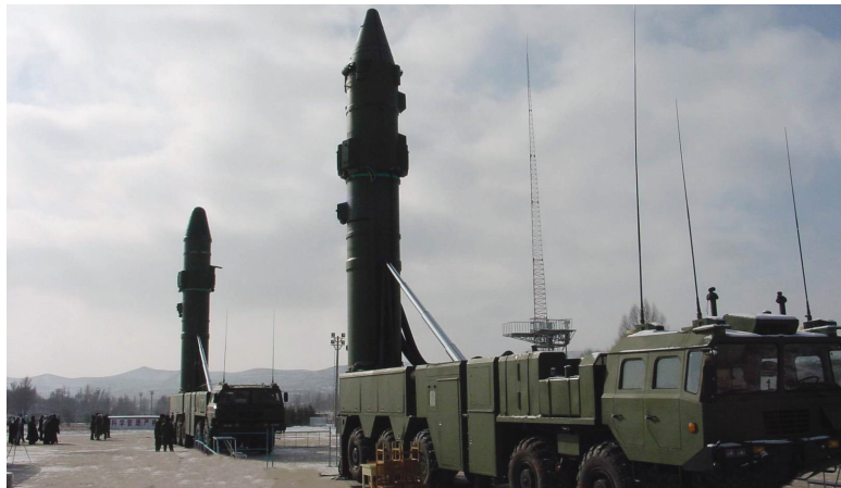
China is developing an ASBM, which could pose a serious threat to U.S. carriers, based on the "D" variant of the CSS-5/DF-21 MRBM. Two different DF-21 variants on transporter erector launchers are pictured here. The missile on the right appears to be a DF-21C while the Office of Naval Intelligence terms the one on the left a "new" variant. Its presence suggests that China's Second Artillery Corps is actively developing additional DF-21 variants.
