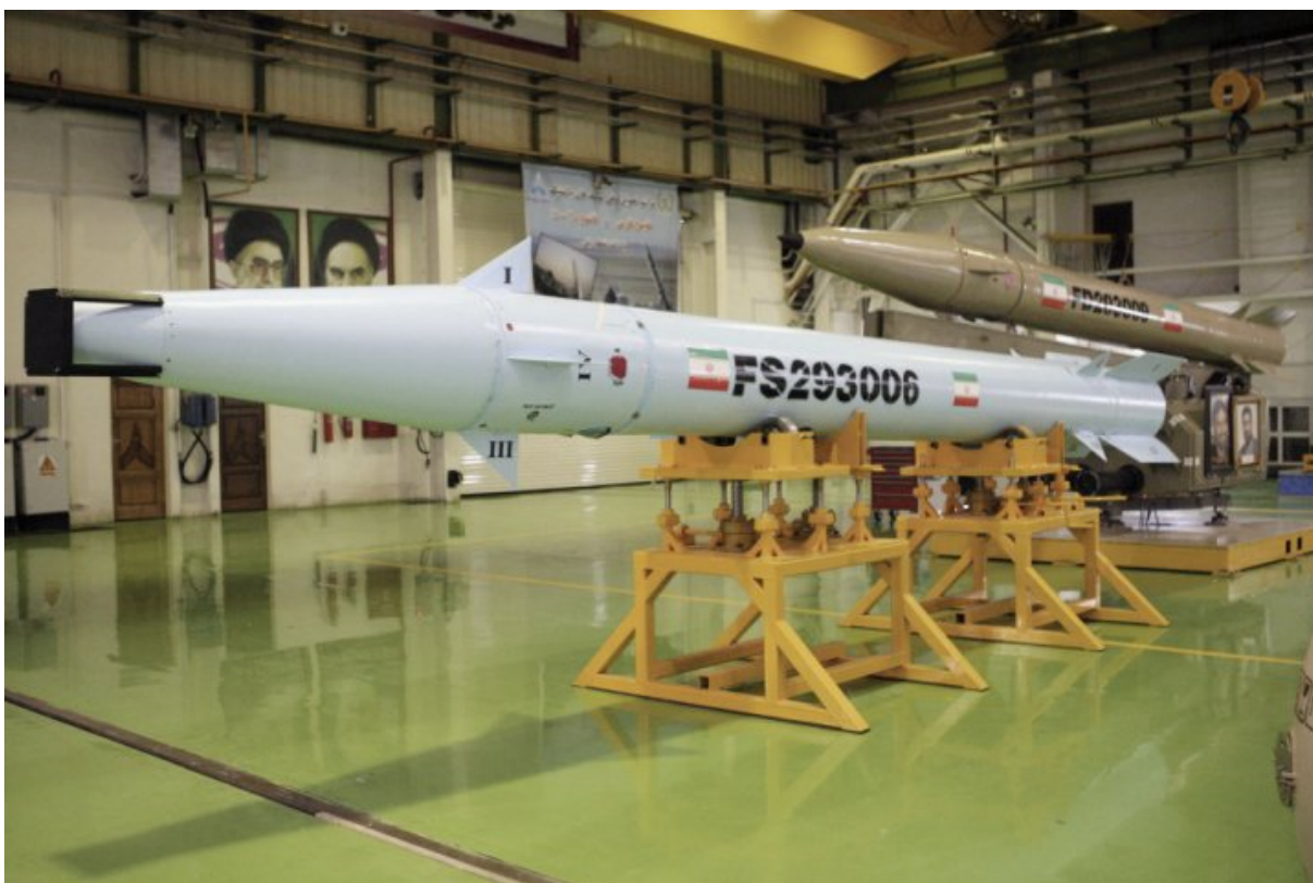
A 2014 picture of what is understood to be Iran's Khalij-e Fars anti-ship ballistic missile, in front of the Fateh-110 short-range ballistic missile from which it was derived. The EO-guided ASBM has fins and canards to enable manoeuvre and could theoretically achieve sufficient in-flight correction to strike a moving maritime target. (Iranian Defence Ministry)
